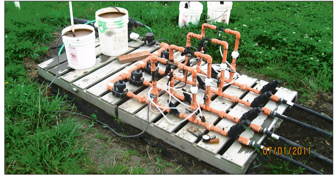
Figure 14. Organic fertilizer pre-mixed in buckets and injected into drip irrigation lines. Photo by Jonathan Roozen.
