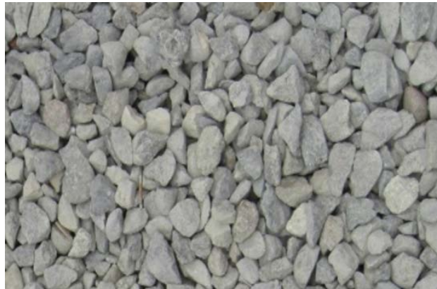
Example of aggregate with fractured, angular faces to allow for a solid and permeable base/reservoir Photo provided by MIG | SvR
